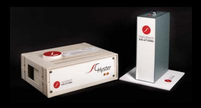
The **Sens AC Hyster™** system is an automate magnetometer that allows to select single or several field conditions for programming individual or multiple magnetization measurements in short times (< 3 minutes). The system generates alternating magnetic fields at three different frequencies ranging from 10 to 100 KHz and field intensities up to 32 kA/m.
