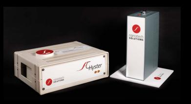
The **Advance AC Hyster™ system** is an automate magnetometer that allows to select single or several field conditions for programming individual or multiple magnetization measurements in short times (< 3 minutes). The system generates alternating magnetic fields at eight different frequencies up to 350 KHz and field intensities up to 24 kA/m.
