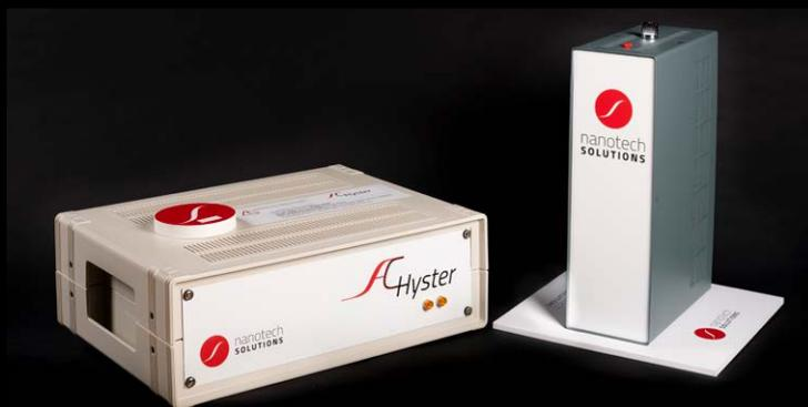
The **LF AC Hyster system** is an automate magnetometer that allows to select single or several field conditions for programming individual or multiple magnetization measurements in short times (~5 minutes). The system generates alternating magnetic fields at single frequency ( $\approx 1$  kHz) and field intensities up to 150 kA/m.
