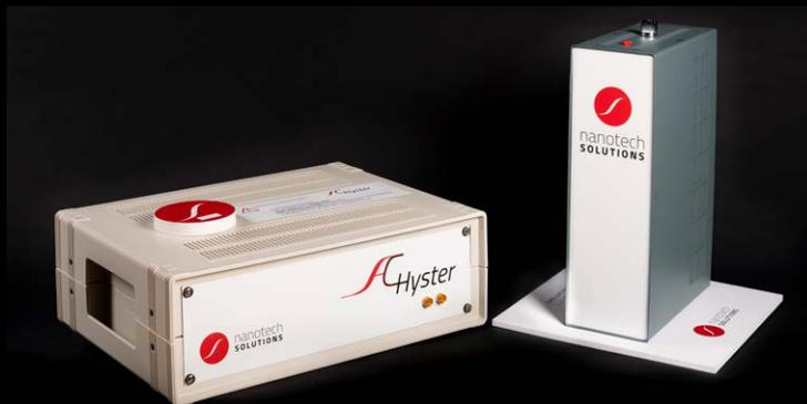
The **Advance AC Hyster system** is an automate magnetometer that allows to select single or several field conditions for programming individual or multiple magnetization measurements in short times (< 3 minutes). The system generates alternating magnetic fields at eight different frequencies up to 350 KHz and field intensities up to 24 kA/m.
