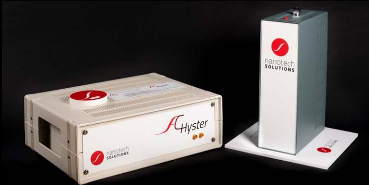
The **Sens AC Hyster** system is an automate magnetometer that allows to select single or several field conditions for programming individual or multiple magnetization measurements in short times (< 3 minutes). The system generates alternating magnetic fields at three different frequencies ranging from 10 to 100 KHz and field intensities up to 24 kA/m.
